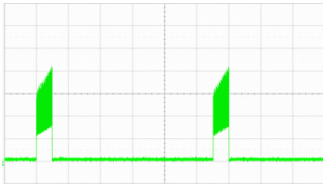
Locked rotor current @ 24 V ( I = 200\text{mA/div} ; t = 1\text{s/div} )
