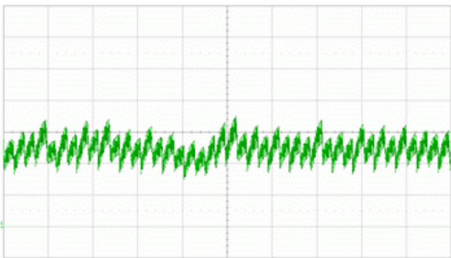
Running current at 48,0 V; 7.000 1/min; I=500mA/Div, t=2ms/Div
