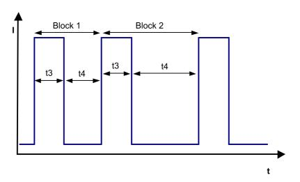
Block1: special locked rotor protection: 5 cycles t3 / t4 = 0,6 s / 1 s Block2: locked rotor protection t3 / t4 = 0,6 s / 10 s
