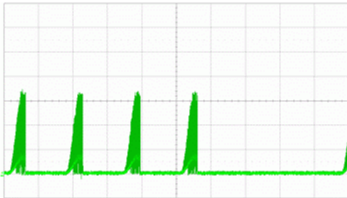
Locked rotor current @ 48 V ( I = 500\text{mA/div} ; t = 10\text{s/div} )
