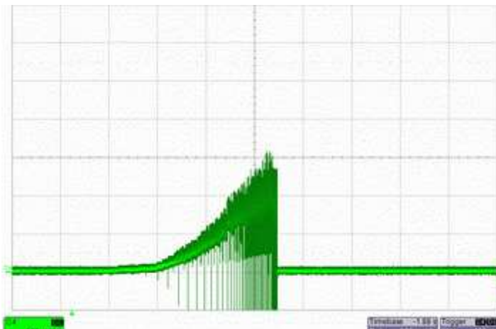
Locked rotor current @ 48 V (I = 500mA/div ; t = 500ms/div)
