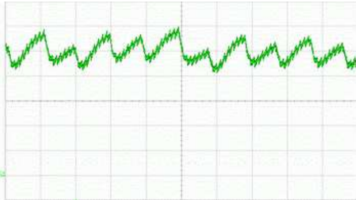
Running current @ 24 V (I = 500mA/div ; t = 500us/div)
